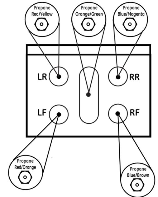
To prevent leakage, make sure the orifices are securely screwed into the gas supply tubes.
